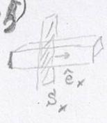
$S_x$  cross-section of the wire at  $x$
