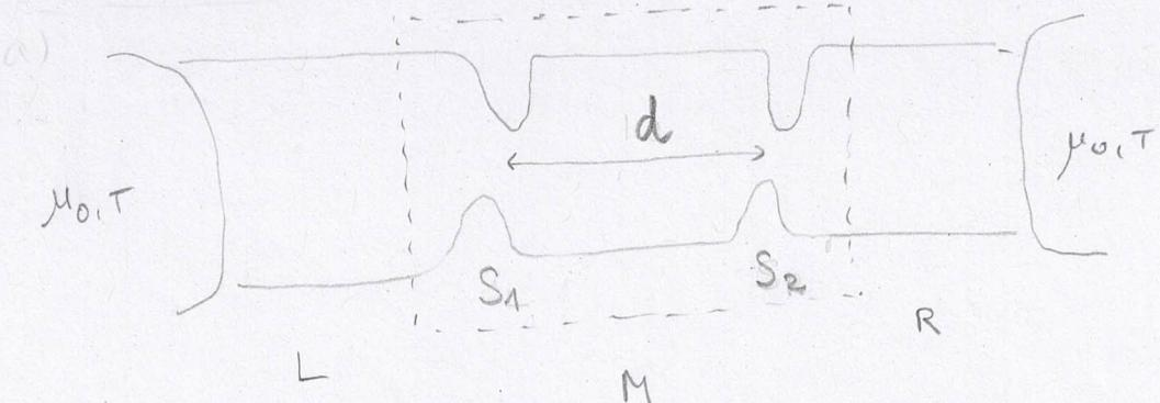
Similar to the situation of the single QPC, the constrictions are well inside the mesoscopic system. Similar to before, if  $V_{ee}$  can be neglected, we can use the Landauer approach and use the Ansatz (4.35) for the traveling states.
