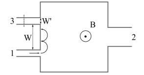
Contact 3 is a voltage probe, contact 1 and 2 serve as source and drain.
